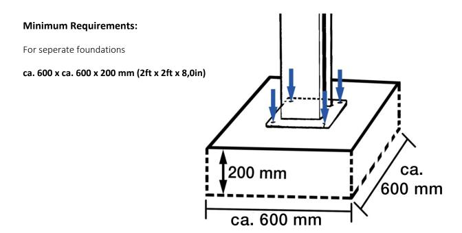
The base plate must be at **least 320 mm larger** in length and width than the post lift above the base plates.
