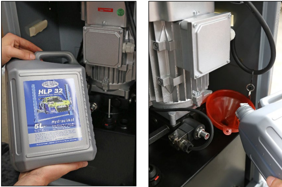
Illustration: Filling with HLP 32
