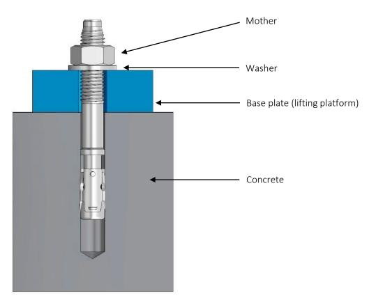
The tightening torque of the anchor bolts (M16) is: 100-110 Nm.
