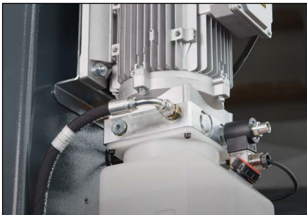
Illustration: Connection of the hydraulic hose
