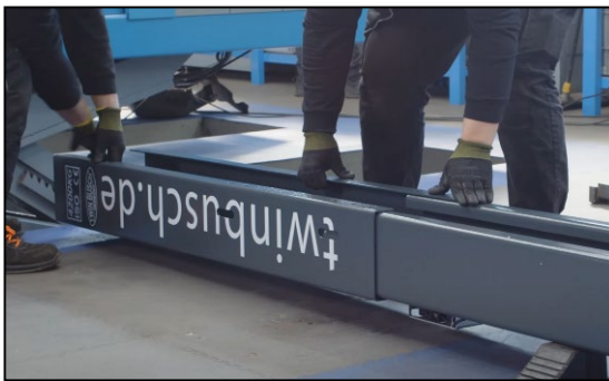
Illustration: Fastening the column extension
