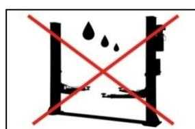
Protect the lift from moisture! Electrical connections must be dry!
