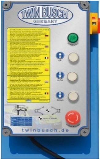
Fit the control unit or control box to the main pillar.
