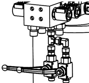
Levelling valve closed
