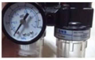
It is recommended to fill the oil tank with ISO VG32 mechanical oil. Set the oil quantity using the knob on the top of the oil tank.
