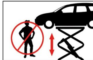
It is forbidden for persons to stand under the lifting platform (when lifting and lowering)!
