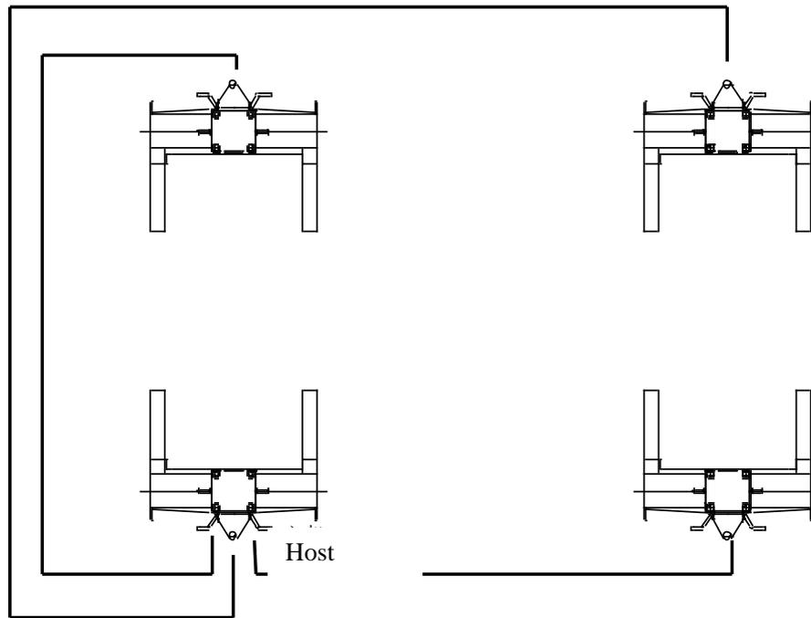
Connection diagram of cables of main and secondary vertical posts (1)
