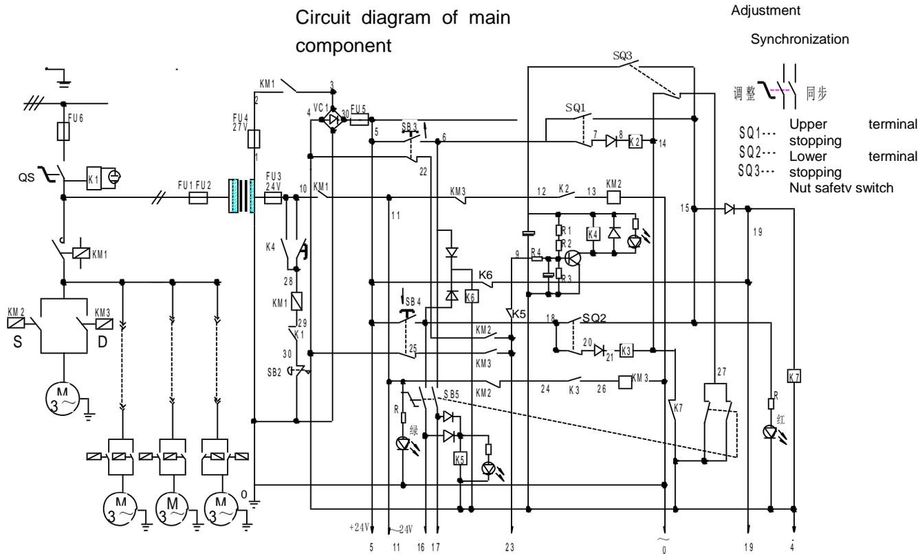
Figure 10 Circuit diagram of main cabinet
