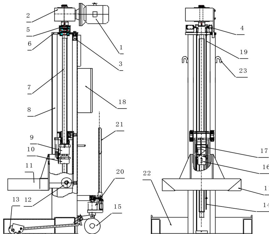
**Figure 3 Structure drawing of vertical posts**
