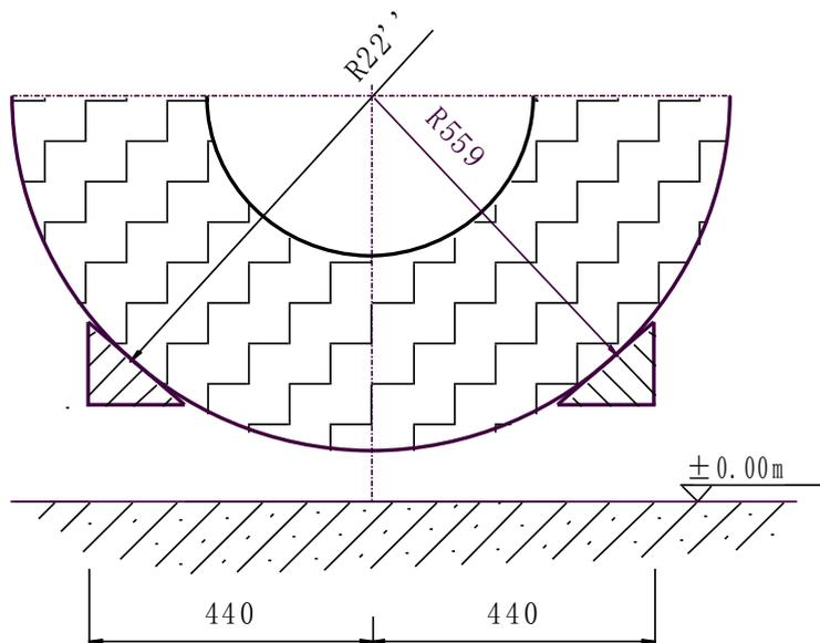
Sketch map for contact of forklift and tire when lifting
