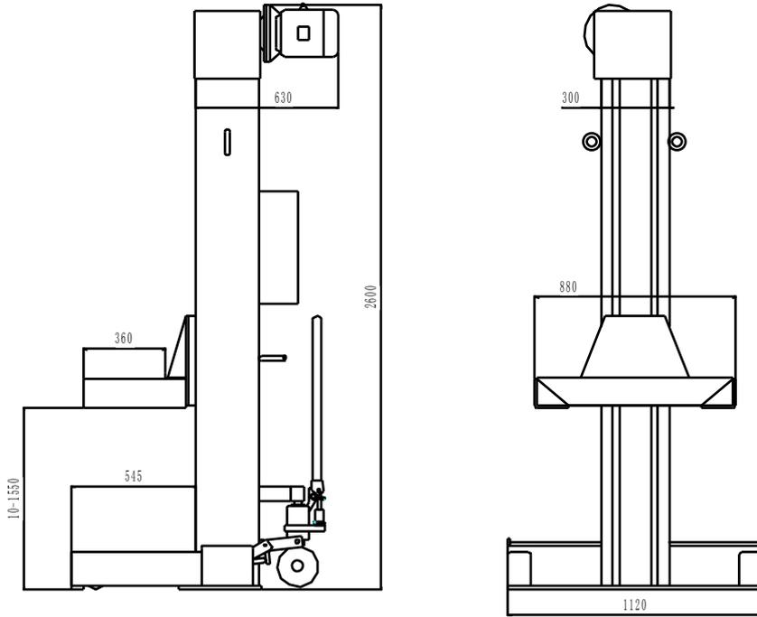
Figure 6 External dimensions of 5.5t vertical post
