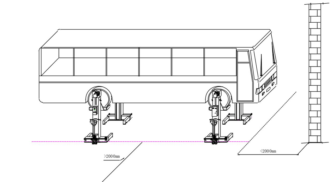
**Figure 17 Sketch map for working area required**
