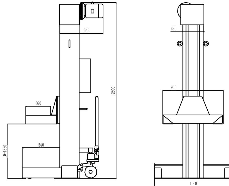
Figure 7 External dimensions of 7.5t vertical post
