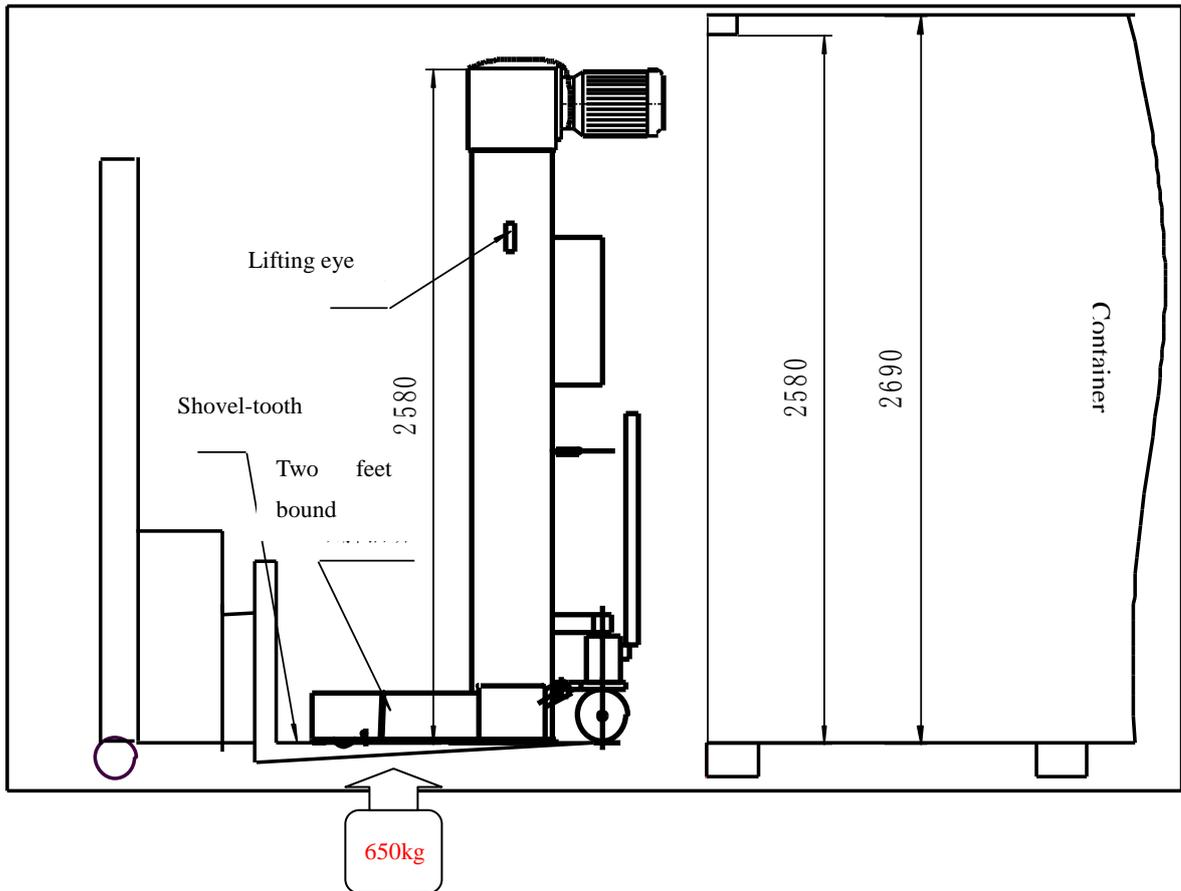
Figure 1 Sketch Map for Lifter's Placement in Container
