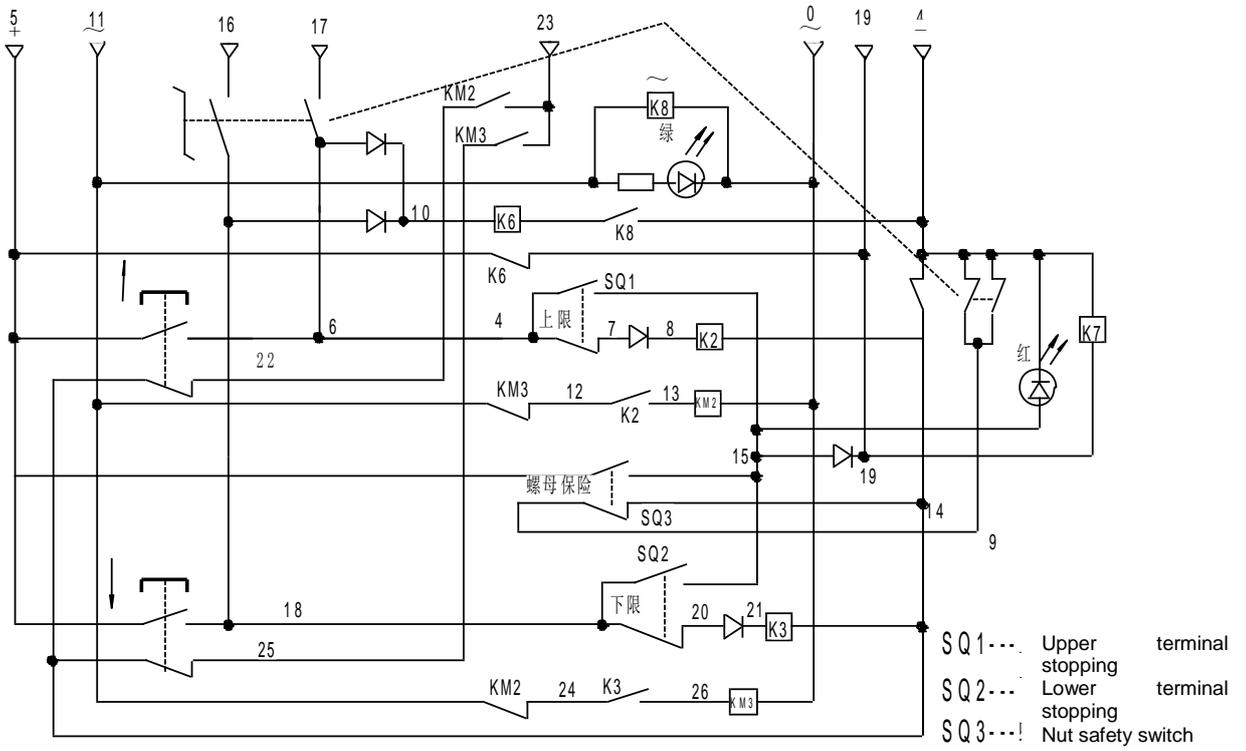
Figure 11 Circuit drawing of secondary control box
